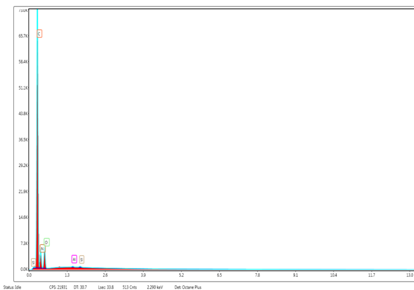
Figure (14): Elements composing the thermally stabilized acrylic nanofiber sample.
