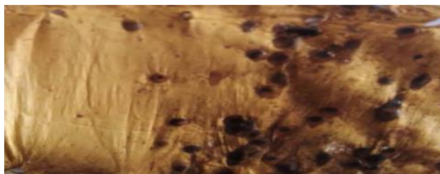
Figure (4): Sample resulting from the thermal stabilization process of the prepared fiber network.
