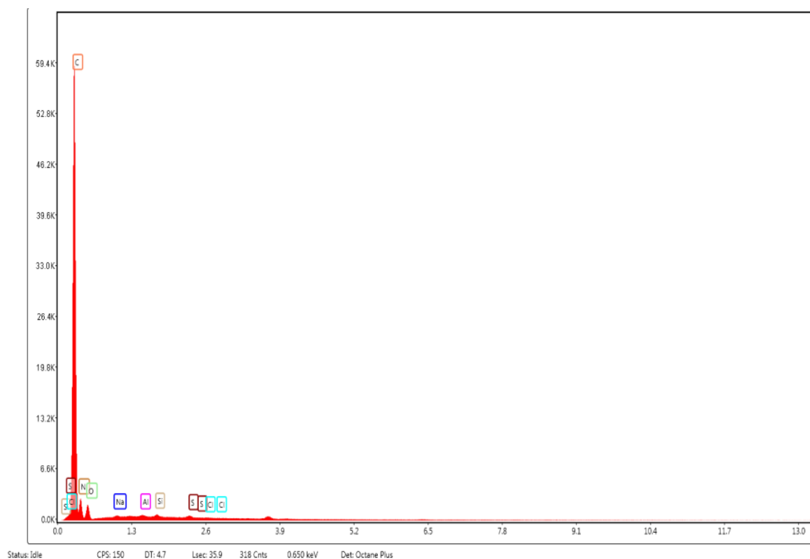
Figure (12): Elements composing the acrylic nanofiber sample.
