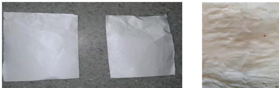
Figure (3): Samples resulting from the electrospinning process of the acrylic solution.
