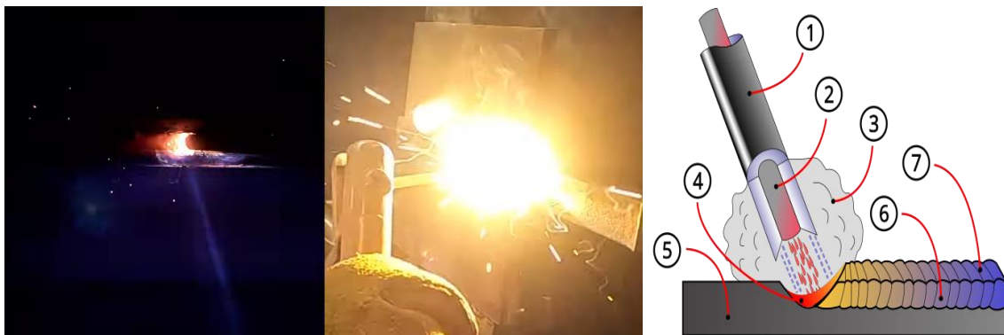
Figure 5: Gas Metal Welding.
