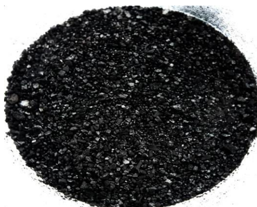
Figure 2. As-prepared green-synthesized nickel oxide nanoparticles (NiO NPs).
