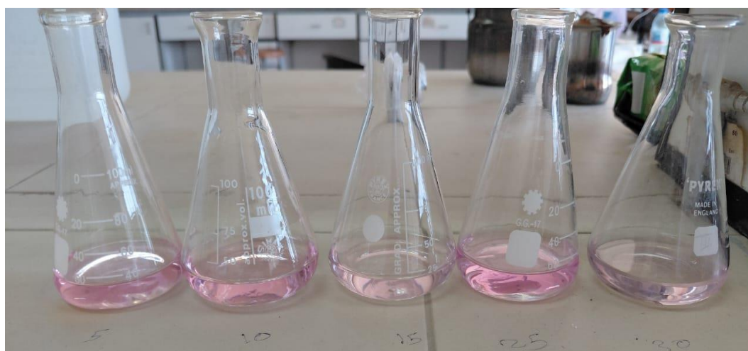
Figure 4. Color change of the reaction mixture at the endpoint of \text{KMnO}_4 titration.
