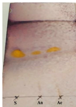
Figure 5: Results of TLC analysis test for unexpired and expired diclofenac sodium coated tablets (Brand A). (S: diclofenac sodium standard, n: unexpired, e: expired).
