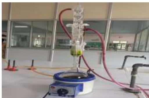
Fig. 3: Figure showing soxhlet extraction of herbs.
