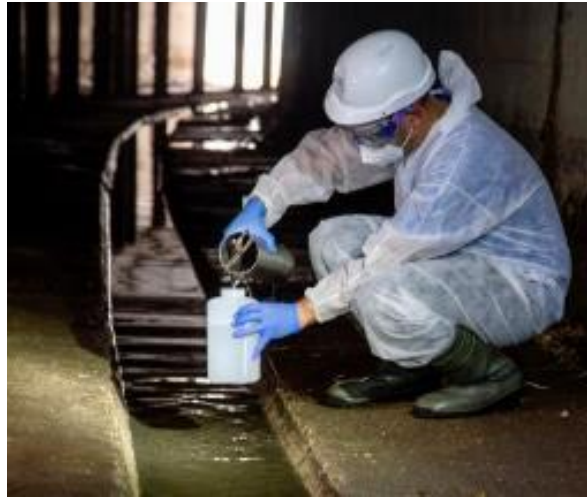
Figure 1: Collection of samples for analysis in wastewater.
