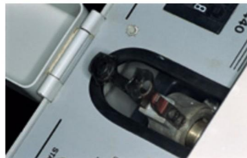
Figure 3. Internal floor surface of amalgamator (assuming no defective open seam) has collected scrap amalgam and beads of elemental mercury. Over time, amalgamators become contaminated to the degree of a biohazard. They represent a source of mercury vapor for dental personnel.
